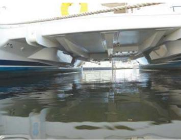
The large aft berths protrude into the tunnel and will pound badly. Bridgedeck clearance is poor. The narrow hulls are overloaded, submerging the transoms (note anti-fouling inside the transoms) and reducing the clearance even more. Aft deck extends to transoms. BCR: 3
