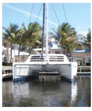
This vessel (empty, at dealer's dock) displays reasonable clearance. Some will be lost when she is loaded, especially as the designer has kept the waterline hull beam narrow for speed; hopefully the chine will not be too noisy. BCR: 7
