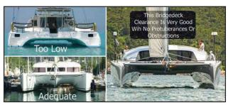
Above: A higher clearance produces less slamming. My rule of thumb is: 4% of the overall length is low, 5% is acceptable, and 6% is good.
