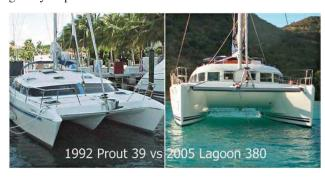
Above: The 2005 38-ft. Lagoon is much bigger in volume and has a much higher bridge deck clearance than the 1992 Prout 39.
