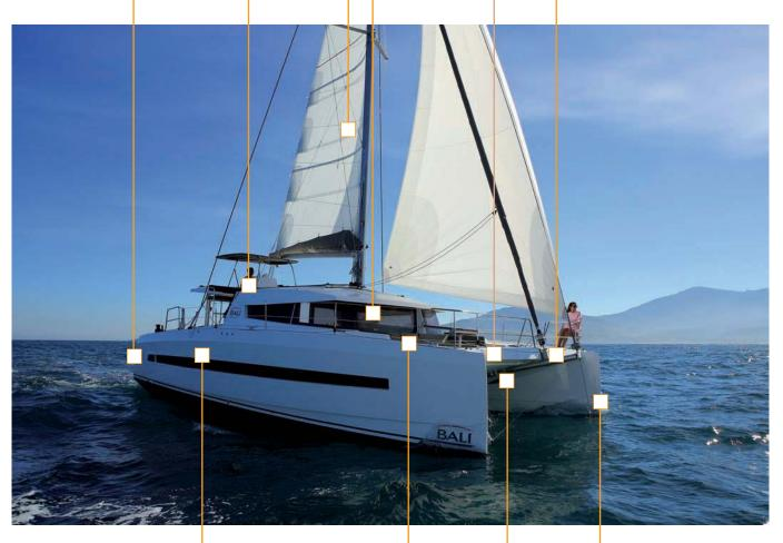
The design of the hulls is elegant and functional; overhang, stepped section and omega profile at the hatches (installed in recesses, allowing them to be left open during squalls), help stiffen the hull sections
