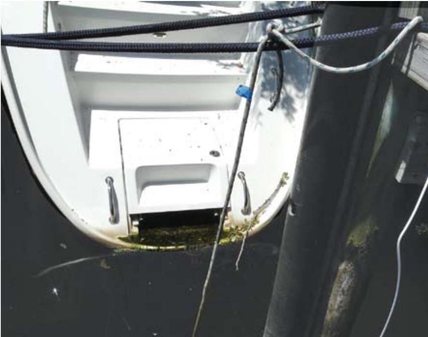
This is an empty boat at the dealer's dock. The built displacement is heavier than the designed displacement. The result is less bridgedeck clearance than the designer intended, transom drag and a fouling problem. Where will the waterline be when it is loaded up to go cruising?
