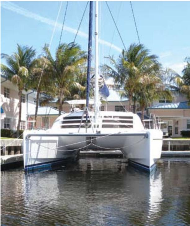
This vessel (empty, at dealer's dock) displays reasonable clearance. Some will be lost when she is loaded, especially as the designer has kept the waterline hull beam narrow for speed; hopefully the chine will not be too noisy. BCR: 7
