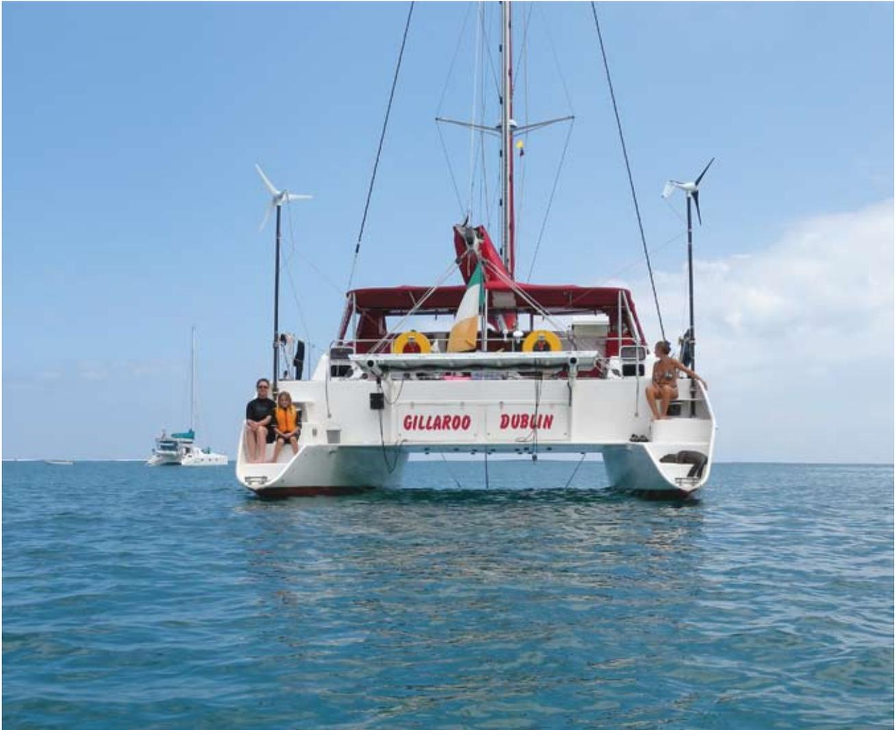
Note the good clearance (33 inches) on this 48-foot catamaran. The bridgedeck is short, the tunnel is completely clean, the hulls have a good length-to-beam ratio (i.e. they are not fat), and the transoms are out of the water, even when loaded for cruising. BCR: 9
