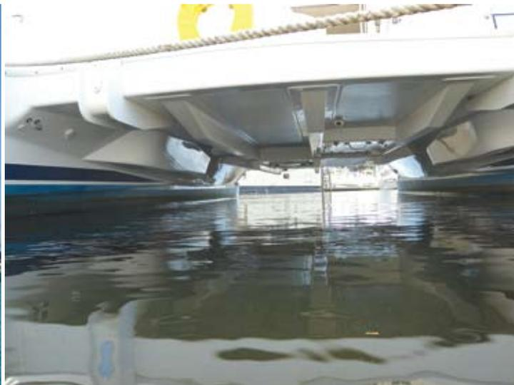
The large aft berths protrude into the tunnel and will pound badly. Bridgedeck clearance is poor. The narrow hulls are overloaded, submerging the transoms (note anti-fouling inside the transoms) and reducing the clearance even more. Aft deck extends to transoms. BCR: 3
