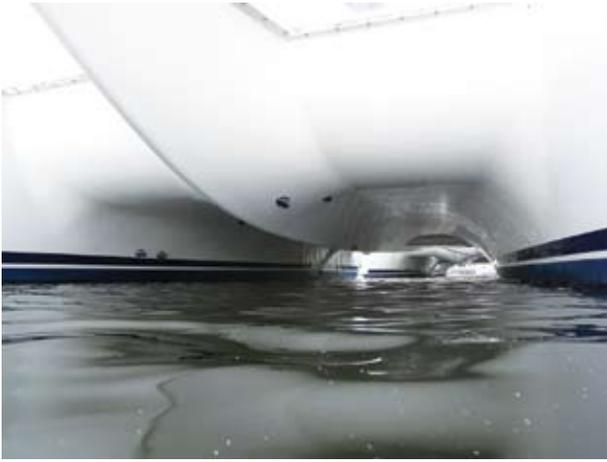
No protuberances, but some serious problems here. Bridge deck clearance is very inadequate; nacelle is too low; leading edge of bridge deck has a large surface area at 45 degrees. On-coming waves will be perpendicular to this surface. BCR: 2
