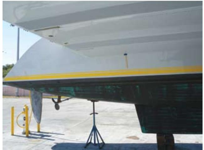
Another large catamaran. Viewed from the bows or the stern, she is a very sleek vessel. The designer has kept the bridgedeck short at both bows and stern, and the tunnel clean. However, when I measured the clearance, it was only 20 inches, which is very disappointing on a beamy, 60-foot vessel. BCR: 6
