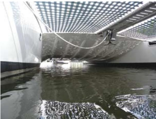
Woefully inadequate clearance, thankfully mitigated by the bridge deck's low profile leading edge, which starts well aft, and no protuberances. BCR: 3
