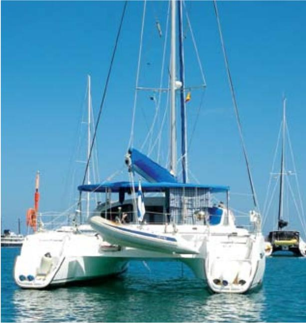
This bridgedeck is high; it stops well short of the transoms. The shelves protruding into the tunnel are small and angled underneath. The transoms are out of the water at loaded displacement. BCR (Bridgedeck Clearance Rating, explained below): 8
